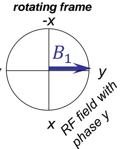
**New:** Direction of  $B_1$  in rotating frame is determined by the initial phase of the RF pulse, it can therefore be changed at our will
