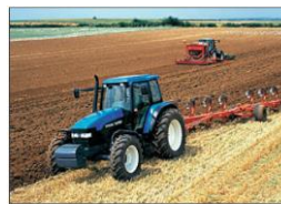
Driving heavy tractors on the subsoil during ploughing and harvesting is a major cause of subsoil compaction. The picture clearly shows how the wheels on one side of the tractor are driven in the plough furrow and press directly on the subsoil (LJHWDA).
