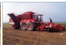
Areas degraded by soil compaction are increasing because wheel loads in agriculture are still increasing. Twenty years ago wheel loads of 50 kN (5000 kg) were considered very high. Nowadays wheel loads of up to 120 kN are used during the harvesting of sugar beet. Modern self-propelled slurry tankers with injection equipment with wheel loads of 90 – 120 kN are used in early spring on wet soils. Large tyres with an inflation pressure of about 200 kPa are needed to carry such high wheel loads. Even on moderate strong soil, compaction of up to 80 cm below the surface have been measured under such loads. The result is that the soil is increasingly compacted to ever-greater depth. The conclusion is that European soil is more threatened than ever (LJHWDA).
